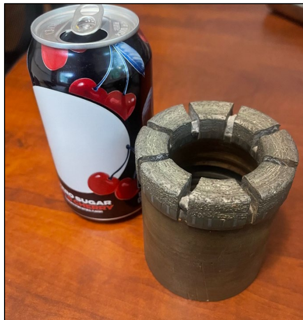
Figure 2.1-3. Diamond-embedded drill bit next to a standard soda can
